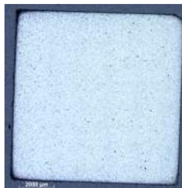
Figure 6 Optical micrograph of sintered component (un-etched)
